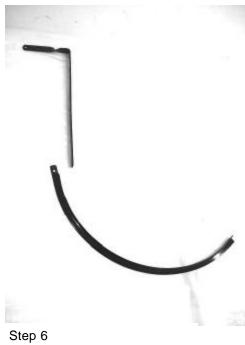
6. Insert # 710232501 Side Arm into wide hem at right rear of the Motor Cover. Attach the Side Arm to the Yoke using a 3/8x1 1/2" hex bolt and wing nut. Place the bolt head on the bottom and nut on the top of the assembly. Mark the fender at the hole in the side arm and drill a 13/32" hole in the fender. Attach the Side
